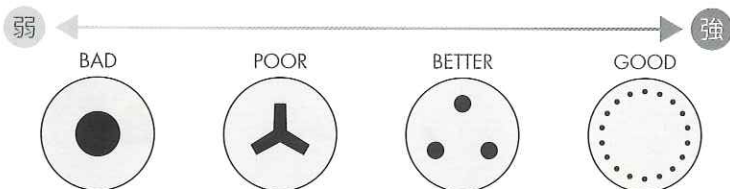
Fig. 1291. Four methods distributing approximately same amount of reinforcing metal. (Form Lakermange, R., and Gonon, P.: J. Am. D. Club Paris 2:1, 1934.)
